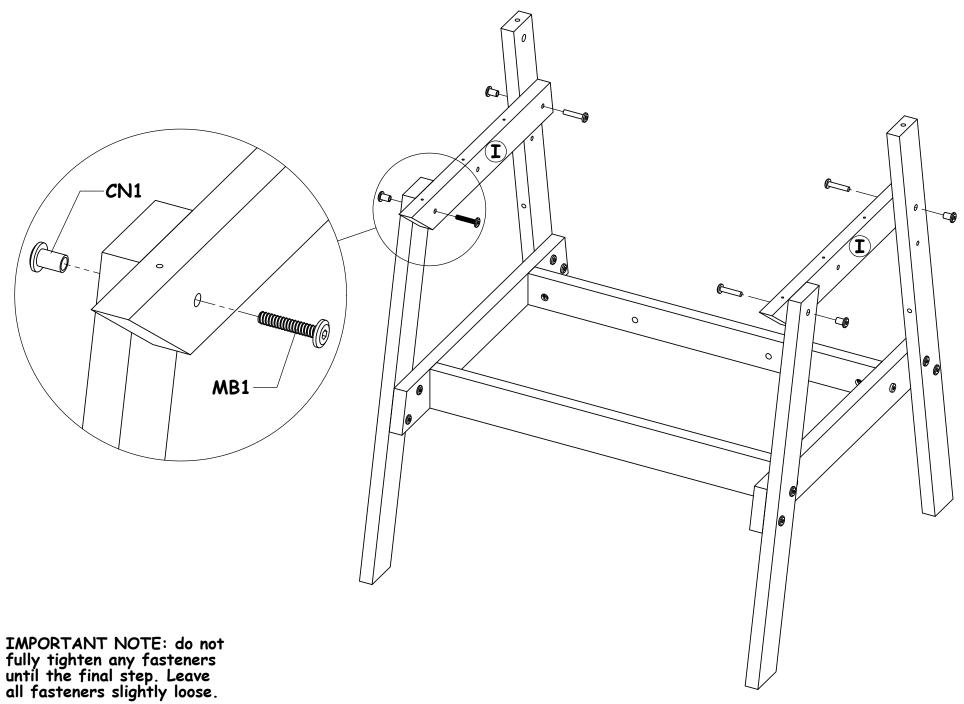
Use 4- MB1 bolts and 4- CN1 nuts to attach upper sides to legs
